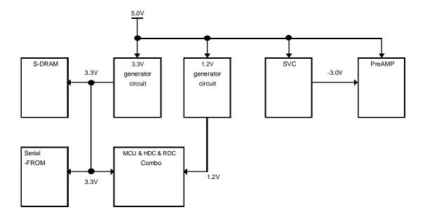
Figure 4.1 Power supply configuration
